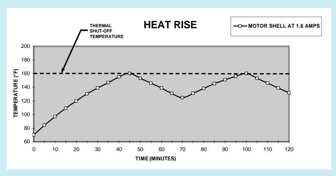
The Aquajet 550 Series Pump is capable of sustaining continuous running for approximately 45 minutes, as shown in the above Heat Rise graph. The motor is equipped with an auto reset thermal protector that will shut down the system, allowing the components to cool. After approximately 25 minutes the pump will restart.
