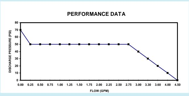
PERFORMANCE MEASURED WITH FLOODED INLET (0 PSI), 70°F (21°C) AMBIENT AND WATER TEMPERATURE, AND VOLTAGE CONTROLLED AT 115 VAC. FLOWS WERE RECORDED AFTER TEMPERATURES HAD STABILIZED. POSITIVE INLET PRESSURE WILL INCREASE THE MAXIMUM FLOW AT THE REGULATED DISCHARGE PRESSURE. MAXIMUM INLET PRESSURE IS 60 PSI.
